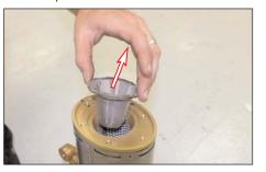
5. Vigorously brush spark arrestor screen with a wire brush to remove accumulated residue.
