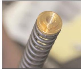
13. The brake-side fork leg goes on the rider's left. Grease up the fork springs, and then re-insert the fork legs into the upper fork tubes, then reinstall the bolts on the top of the triple clamp and screw them into place, making sure that the notch on the top of the fork internals is pointing inward toward the opposite fork leg. Be prepared to hold the bottom of the fork leg in place in order to tighten the top bolt completely.
