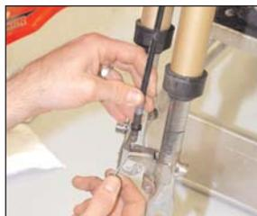
6. Remove the front-brake cable from the front-brake lever.
