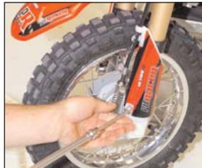
3. Using 14mm and 19mm wrenches, remove the front wheel and remove the front axle.
