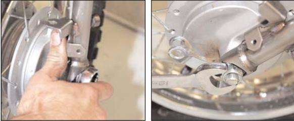
21. Adjust the brake cable to the desired tension.
