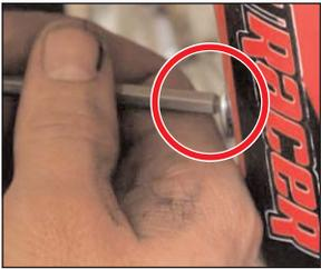
19. Take the supplied longer front-brake cable, and then route the end with the notch on the cable back into the front-brake lever.
