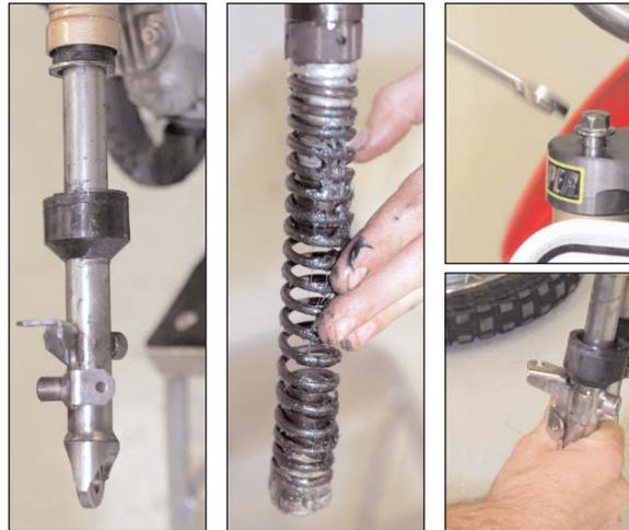
14. Next, reinstall the circlips just like you found it to begin with, and then use an open ended wrench to push it into place until it makes an audible clicking noise.
