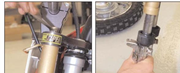
8. Remove the rubber boot that sits in the junction between the lower and upper fork legs, then use a rag to clean out the dirt and grease inside the bottom of the top fork leg. After that, use the snap-ring pliers to remove the circlip from inside the area you just cleaned out. The rest of the fork and its internals will come out with the circlip.
