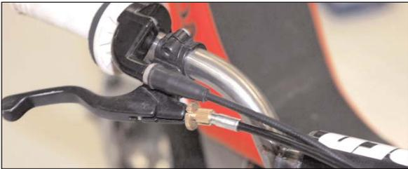
20. Route the bottom end of the brake cable through the fork guard and then through the top tab on the fork tube. Then replace the spring you removed in Step 4, route the threaded end through the tab on the brake assembly, and then replace the wing-nut to hold the brake in place.
