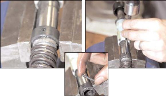
10. Slip the new spring into the bushing as shown below, making sure to line up the holes in the bushing, fork tube and gold spring end.
