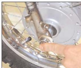
4. Loosen the wing-nut on the bottom of the front-brake assembly, as shown. Make sure not to lose the spring, which is likely to bounce away somewhere if you're not careful.
