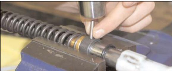
12. Keep in mind, when you put the fork internals back into the fork tubes, the notches on the top of the internals point toward each other in the front end of the bike.
