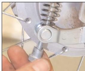
5. Remove the brake cable from the left fork leg.
