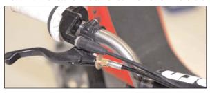
20. Route the bottom end of the brake cable through the fork guard and then through the top tab on the fork tube. Then replace the spring you removed in Step 4, route the threaded end through the tab on the brake assembly, and then replace the wing-nut to hold the brake in place.
