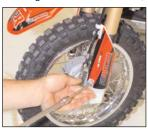
3. Using 14mm and 19mm wrenches, remove the front wheel and remove the front axle.
