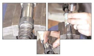
10. Slip the new spring into the bushing as shown below, making sure to line up the holes in the bushing, fork tube and gold spring end.
