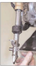
15. Slide the rubber boot back up over the junction between the bottom and top of the fork leg.
