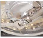
18. Re-install the fork guards using a 5mm Allen wrench.
