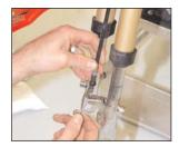
6. Remove the front-brake cable from the front-brake lever.
