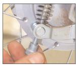
5. Remove the brake cable from the left fork leg.
