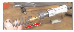
11. Hammer the pin back into the hole, making sure it's recessed below the bushing because you don't want it scraping the sides of the fork tube. Repeat starting for the other fork leg.
