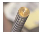
13. The brake-side fork leg goes on the rider's left. Grease up the fork springs, and then re-insert the fork legs into the upper fork tubes, then reinstall the bolts on the top of the triple clamp and screw them into place, making sure that the notch on the top of the fork internals is pointing inward toward the opposite fork leg. Be prepared to hold the bottom of the fork leg in place in order to tighten the top bolt completely.
