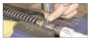
12. Keep in mind, when you put the fork internals back into the fork tubes, the notches on the top of the internals point toward each other in the front end of the bike.
