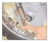
Loosen the wingnut on the bottom of the front-brake assembly, as shown. Make sure not to lose the spring, which is likely to bounce away somewhere if you're not careful.
