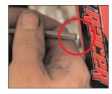
24. Take the supplied longer front-brake cable, and then route the end with the notch on the cable back into the front-brake lever.
