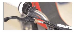
25. Route the bottom end of the brake cable through the fork guard and then through the top tab on the fork tube. Then replace the spring you removed in Step 4, route the threaded end through the tab on the brake assembly, and then replace the wingnut to hold the brake in place.
