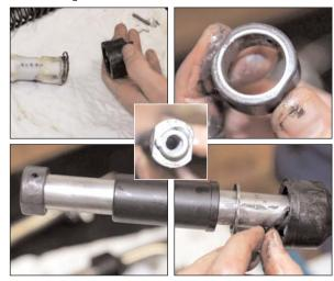
16. Then hammer the pin back into the hole, making sure it's recessed below the bushing because you don't want it scraping the sides of the fork tube. Repeat starting at 10 for the other fork leg.
