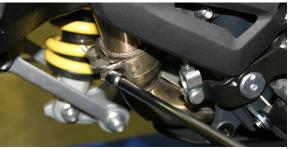
4. Remove stock muffler assembly.
