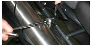
Loosen pipe joint clamp.
