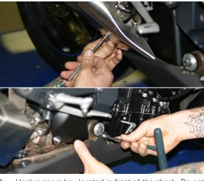
Unplug servo box located in front of the shock. Do not turn ignition on while servo is unplugged.
