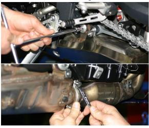
8. Remove OEM muffler assembly and servo box.
