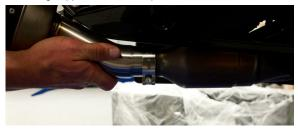
15. Attach muffler clamp to foot peg mount using stock bolt and washer with supplied 8mm flange nut.
