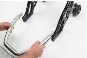
Use supplied 8x25mm socket head flat bolts and tighten to 15 ft-lbs.
