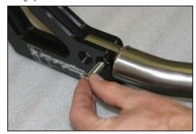
5. Use supplied 8x25mm socket head flat bolts and tighten to 15 ft-lbs.
