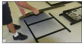
3. Set lower back support on lower stand plate and mount with 2 8x55mm bolts.
