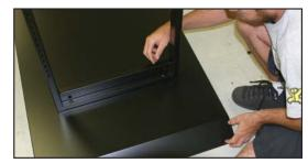
Install center support and secure in place with 8x55mm bolt into lower stand plate and 8x45mm bolt between back support and center support.
