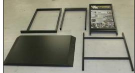
Locate lower stand retainer and plate, set lowerstand plate over retainer and line-up mounting bolts.
