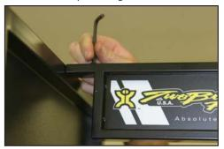
7. Install exhaust display using the 2 8x15mm bolts/ nuts.
