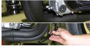
6. Remove O2 sensor from OEM head pipe.
