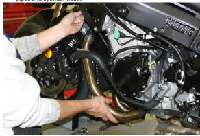
Install the TBR V.A.L.E.™ muffler assembly to slip-on tube using the 4 6x14mm S.H.C.S. and lock washers provided. Leave loose for now.
