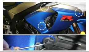
Remove radiator mounting bolts and let radiator sit against front fender.
