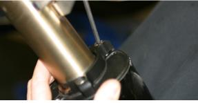
11. Loosely attach muffler to bike using the OEM hardware on slip-tube mount and install muffler clamp using the supplied bolt and spacer.
