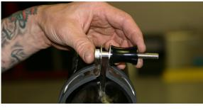
12. Install supplied O2 adapter. Install O2 sensor into O2 adaptor.
