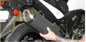
8. Install TBR mid-pipe using OEM mounting hardware and supplied 57mm barrel clamps.
