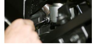
6. Remove heatshield to access muffler mounting bolts. Remove OEM mounting hardware.
