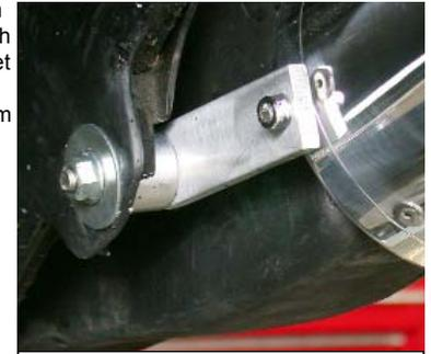
Finished Installation detail (preproduction bracket shown)
