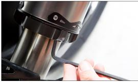
6. Tighten muffler mount and then barrel clamp.
