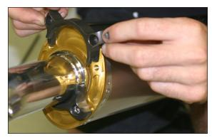
4. Attach barrel clamp to end of slip-tube and slide rubber lined muffler clamp over the exhaust and fit to bike loosely installing the supplied bolt, spacer to the muffler mount and re-use the OEM nut in this order: Bolt > Clamp > Spacer > Mount > Nut.
