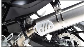
Attach TBR slip tube to TBR muffler using the 2 piece X-Rings and 6x20mm socket head cap screws with lock washer that are provided. Leave loose enough to make some adjustments on the motorcycle.
