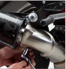
. Before you run the bike, clean off all fingerprints and dirt, as any oily residue will etch the metal and become somewhat permanent when the system gets hot. Also, remove any protective plastic from the name badges on the muffler canister(s) or the muffler clamp(s). Run the bike and enjoy. It is normal for some white smoke to appear the first time you start the bike. This is packing/manufacturing oil from inside the pipe burning off. After 50 to 100 miles, recheck all fasteners for tightness.
