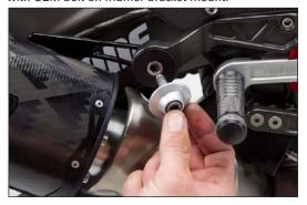
5. Check alignment and then tighten muffler mount bolt and finally barrel clamp.
