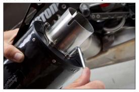
Install TBR muffler assembly to bike, use supplied nut with OEM bolt on muffler bracket mount.
