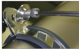
\*a small amount of high temp silicone on slip joint may be used.
