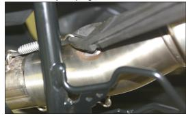
3. Remove muffler mounting bolt and decorative washer, set aside to re-use washer later.
