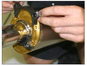
Attach muffler assembly to motorcycle using the OEM springs and suplified muffler clamp. Use the supplied 8x20mm socket head cap screw and OEM washer to secure muffler clamp.
