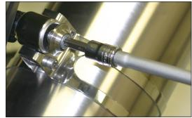
4. Attach TBR slip tube to TBR muffler using the 2 piece X-Rings and 6x14mm socket head cap screws with lock washer that are provided. Leave loose enough to make some adjustments on the motorcycle.
