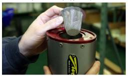
Insert Q1 Quiet Core being sure to fully seat it into the groove in the Billet Outlet Cap. Be sure to align the angle of the Q1 Quiet Insert to the angle of the endcap.
