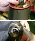
5. Reinstall endcap. Apply threadlock to the gold anodized aluminum bolts and tighten endcap.
