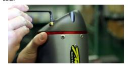
3. Remove the spark arrester (if applicable)
