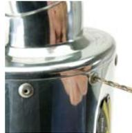
3. Use a rubber/dead-blow mallet to gently tap out the outlet. Tapping on alternate sides will help "walk" the outlet out.
