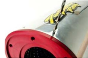
6. Install rivets. The large head rivets (3/8") are for use with aluminum muffler sleeves, the small head rivets (1/4") are for use with carbon fiber, x-metal cf or titanium muffler sleeves. For the carbon fiber, x-metal cf and titanium mufflers, you must also reinstall the reinforcing band with the rivets.
