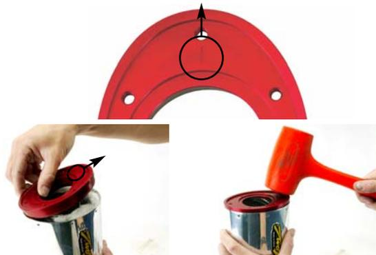
5. Using the existing holes in the muffler sleeve as guides, drill new holes into the billet outlet cap.
