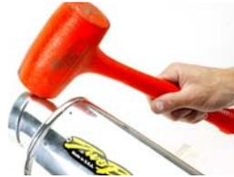
4. Install Billet Outlet Cap (Red) by tapping it into the muffler sleeve. Use a rubber or dead-blow mallet so as not to damage the billet outlet cap.
