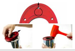
Using the existing holes in the muffler sleeve as guides, drill new holes into the billet outlet cap.
