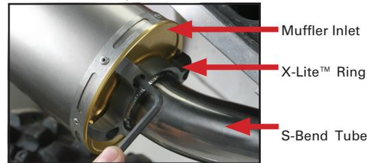
5. Slide the S-bend connector pipe into the end of the headers. Leave loose for now.
