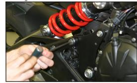
4. Remove muffler mounting hardware.
