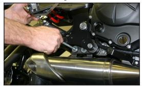
5. Remove header nuts from cylinder head and remove header assembly.
