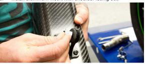
Apply a thin layer of anti-seize to slip tube outlet and connect to muffler with supplied hook springs.
