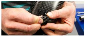
6. Install aluminum insert with shoulder facing out.
