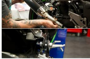
14. Tighten barrel clamp.
