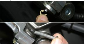
Install Muffler bracket using previously installed 6x45mm bolt and OEM muffler bolt. Use supplied 6mm nylon lock-nut to secure in place.
