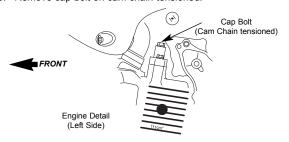
6. Turn the crankshaft counterclockwise until the "T" on the camshaft sprocket aligns with the projection on the head (approx. at 9 o'clock position) and the "T" on the flywheel aligns with the projection on the engine case (approx. at 9 o'clock position).
