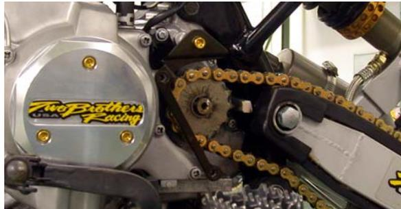
4. Install the new sprocket cover using the remaining supplied bolts. Grease the threads of the bolt and torque to 84 in-lbs.
