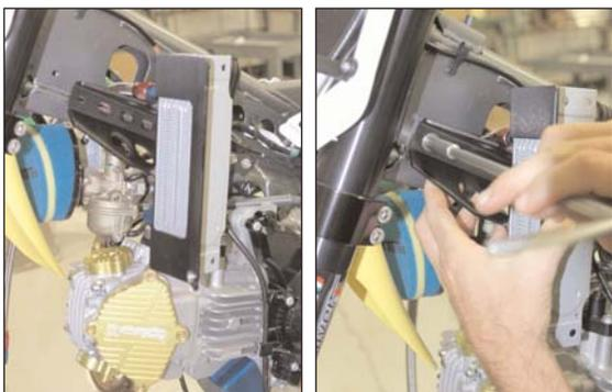
11. Bring both oil lines down behind the head pipe keeping the "lower" line on the left and the "upper" line to the right.
