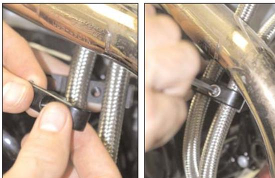
14. Attach the oil line mounting bracket to the engine case using the supplied bolt. Tighten securely.
