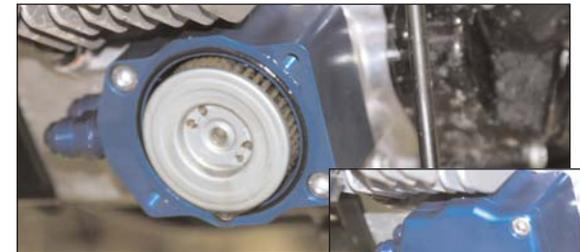
attach filter housing cover. Tighten securely.
