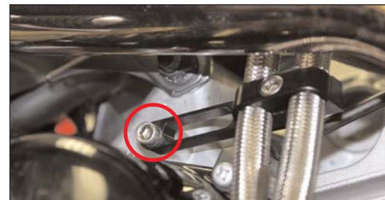
15. Securely tighten the bolt securing the oil lines to the bracket.
