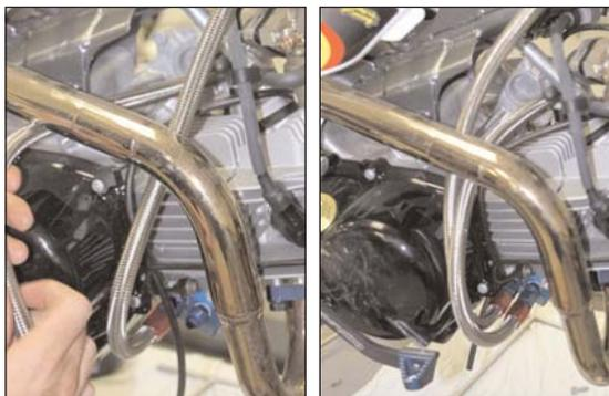
13. Remove the bolt securing the two halves of the supplied oil line retainer bracket. With the mounting hole of the bracket facing rearward, secure the two oil lines into the mounting bracket and replace the bolt. Do not fully tighten.
