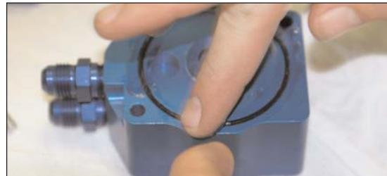
6. Insert the two supplied bolts through the filter housing and attach filter housing to engine case. Tighten both bolts securely.
