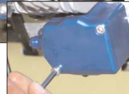
8. Orient the heat exchanger so that the rectangular flange is to the left and the mounting bracket is to the right. Attach the oil line with the right-angle connector to the lower port of the exchanger. Attach the remaining hose to the upper port - it does not matter which end connects to the exchanger. Securely tighten both connections.
