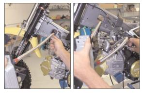
10. Attach the heat exchanger to the frame. Tighten securely
