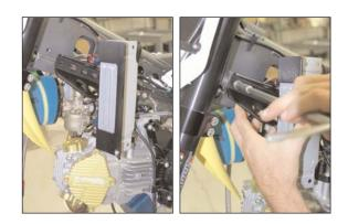
Bring both oil lines down behind the head pipe keeping the "lower" line on the left and the "upper" line to the right.
