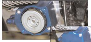
attach filter housing cover. Tighten securely.
