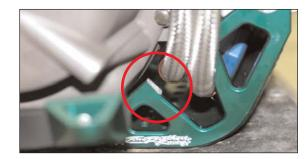
Double check your work and make sure all hardware is securely tightened. After and hour of riding re-check all hardware and tighten if needed.
