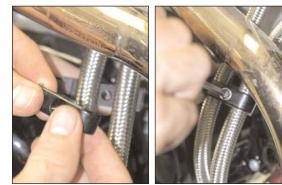
14. Attach the oil line mounting bracket to the engine case using the supplied bolt. Tighten securely.
