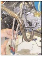
12. Attach the upper line to the rear port of the new filter housing. Tighten securely. Attach the lower oil line to the forward port. Tighten securely.
