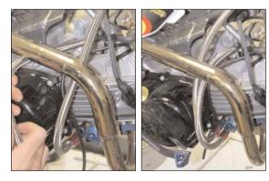
13. Remove the bolt securing the two halves of the supplied oil line retainer bracket. With the mounting hole of the bracket facing rearward, secure the two oil lines into the mounting bracket and replace the bolt. Do not fully tighten.
