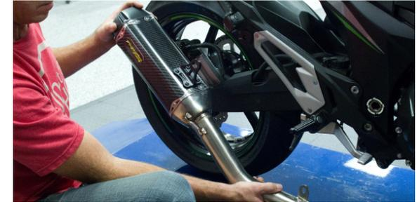
8. Attach TBR muffer system to motorcycle using OEM hardware on lower mount with supplied 10mm nut. Use 8x75mm socket head cap screw and 18mm spacer with 8mm nut on muffer mount.
