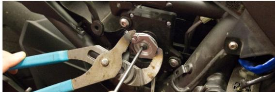
6. Remove OEM muffer mounting bolts and remove from motorcycle.
