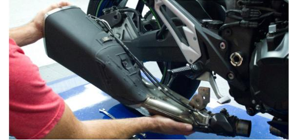
7. Attach TBR slip tube to TBR muffer using the supplied springs.
