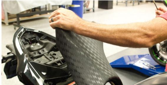
4. Remove body work from right side of motorcycle to access butterfly valve servo cables.
