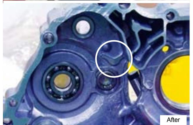
14. Using a dremel(or similar) tool you will need to clearance the inside of the case slightly for the new kickstarter gear. It is best to install the gear first and look at how much material needs to be removed. Please note that not a lot of material needs to be removed in order to gain adequate clearance.
