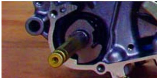
Before installing the shiftshaft assembly you will need to trim it. Cut just beyond the welded area (be sure NOT to cut the weld). Do your cutting BEFORE installing the shiftshaft assembly.
