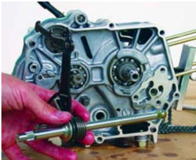
5. Remove the snap ring from the kickstart shaft with snap ring pliers. Remove the kick start spring assembly. Note orientation of this piece, you may wish to practice installation of this piece before proceeding as this will make it easier to do so later on.
