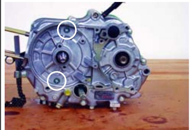
9. Remove the cam tensioner bolt (17mm bolt), then remove the tensioner arm, guide wheel and cam chain.
