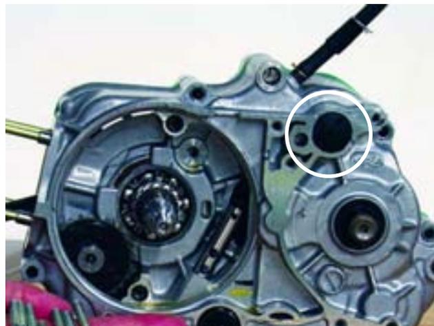
Remove the 10mm shift drum bolt. Now turn the case around and the entire transmission can be removed.
