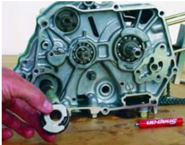
6. Using an impact wrench remove the flywheel nut. If you do not have an impact wrench you can use the Rotor Holder (# 010-9-01-05). Remove the flywheel using the Takegawa Flywheel Puller (# 010-9-01-03) or equivalent.
