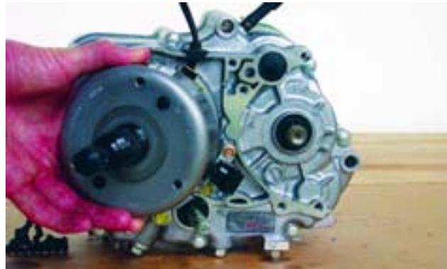
7. Remove the left side engine cover. Remove the magnet assembly (left side of).
