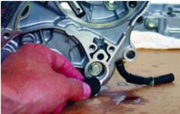
Remove the shift detent piece.
