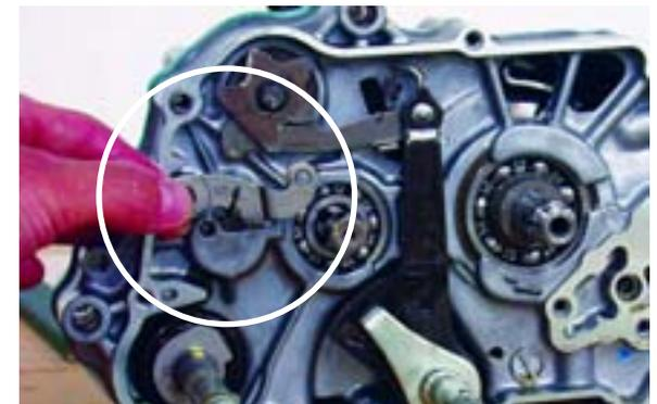
Remove the star shaped piece by removing the 10mm headed bolt.
