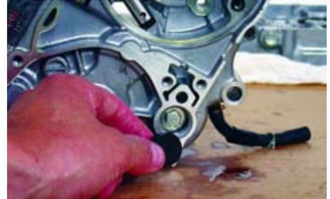
13. For the Takegawa 5 Speed Transmission to work you will need to cut this tab off of the inside of the case.
