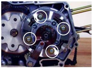
After the cover is removed, you will be able to see the clutch locknut. Peel back the safety tabs and remove the clutch locknut using the Clutch Locknut Tool (# 010-9-01-03) or equivalent. Once this nut is removed slide the stock clutch off.
