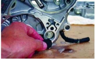
Remove the shift detent piece.
