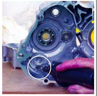
15. Before reassembly, thoroughly clean the cases and bearings being sure to remove all debris. Relube the bearings with an engine assembly lube (be sure to coat the gears as well) and install the Takegawa 5 Speed Transmission
