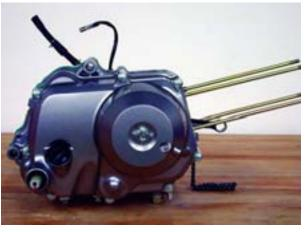
2. Remove the right side engine cover. Remove the clutch by first removing the arm on the shaft, be careful not to lose the spring or the bearing.
