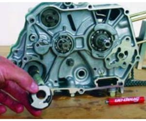
Using an impact wrench remove the flywheel nut. If you do not have an impact wrench you can use the Rotor Holder (# 010-9-01-05). Remove the flywheel using the Takegawa Flywheel Puller (# 010-9-01-03) or equivalent.
