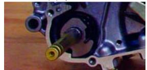
Before installing the shiftshaft assembly you will need to trim it. Cut just beyond the welded area (be sure NOT to cut the weld). Do your cutting BEFORE installing the shiftshaft assembly.
