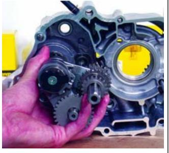
16. Reinstall the 10mm shfit drum bolt and rubber cover. This will keep the transmission in place.
