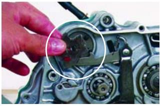
Slide the shaft assembly completely out.
