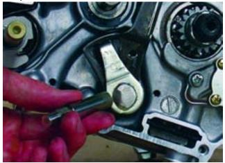
Install the detent arm in the reverse order you disassembled them. Check for proper operation by spinning the shaft by hand, it should spin smoothly.
