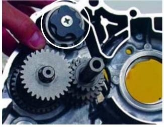
Install the new kick starter gear and spindle (# 010-3-04-001). Check for smooth operation by spinning the transmission. Reinstall the crankshaft and bolt the engine cases back together.
