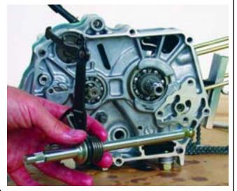
5. Remove the snap ring from the kickstart shaft with snap ring pliers. Remove the kick start spring assembly. Note oriention of this piece, you may wish to practice installation of this piece before proceeding as this will make it easier to do so later on.
