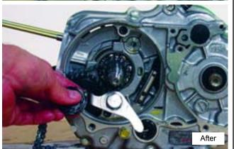
10. Remove the seven 8mm bolts from around the edge of the engine case. Take note of the different lengths.
