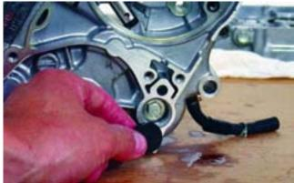
13. For the Takegawa 5 Speed Transmission to work you will need to cut this tab off of the inside of the case.
