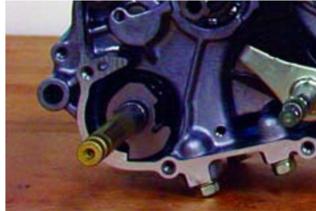
Your new 3 speed has a new shift shaft supplied so you do not have to complete this step, but you will have to use the supplied shifter. **The stock or aftermarket shifter will not work with the supplied shift shaft you will have to use the new shift inconjunction with the supplied shift shaft.**
