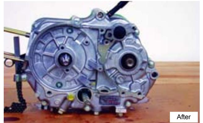
8. Remove the two phillips head screws from the cam chain inner cover. These screws are pretty tight so you may have to use an impact driver to break them loose. Remove the screws and the cover.
