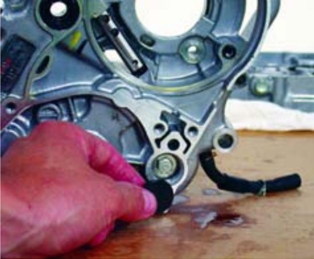
Remove the shift detent piece.
