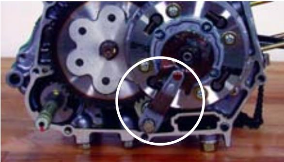
Remove the four phillips head screws and remove the cover.
