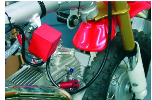
Installed Kit Ignition Coil
