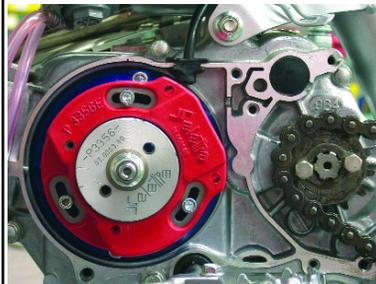
Installed Kit Stator
