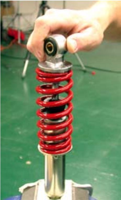
9. Tighten 14mm nut and eyelet the same way it was removed.
