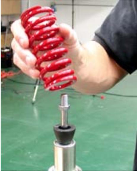
8. Screw top eyelet onto shaft.
