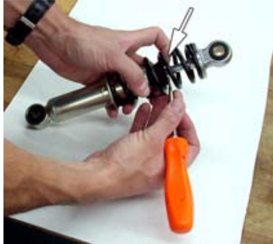
4. Loosen nut with 14mm wrench - will only turn approximately  $\frac{1}{4}$  of a turn.
