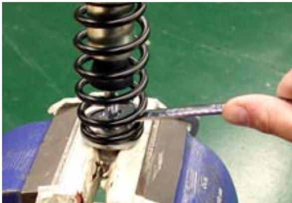
5. Hold the nut secure with the 14mm wrench, slide large screwdriver thru top eyelet and unscrew top eyelet off shock.
