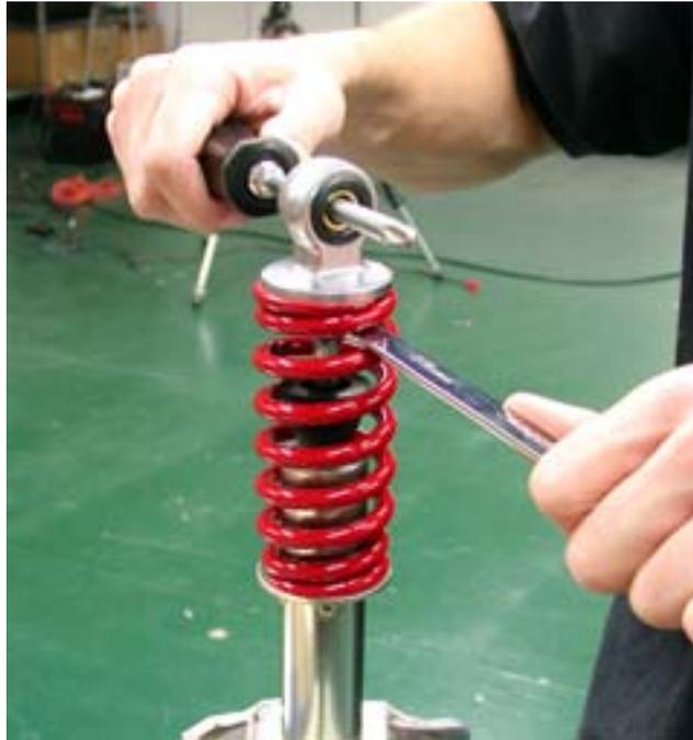
10. Apply a small amount of grease to the top and bottom shock bolts.
