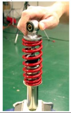
9. Tighten 14mm nut and eyelet the same way it was removed.
