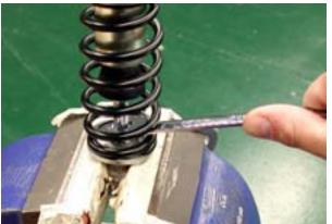
Hold the nut secure with the 14mm wrench, slide large screwdriver thru top eyelet and unscrew top eyelet off shock.
