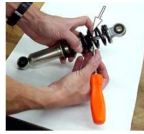
Loosen nut with 14mm wrench - will only turn approximately ¼ of a turn.
