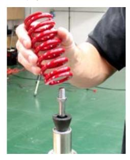
8. Screw top eyelet onto shaft.
