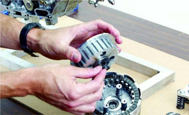
7. Note the order in which the bearing and spacers go over the clutch mainshaft.
