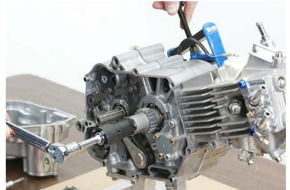
5. Using a hammer and a punch, gently fold over one of the tabs on the lock washer into the clutch bearing slot.
