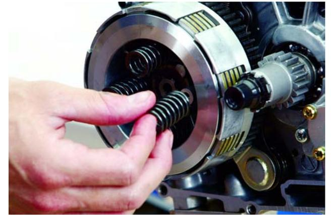
13. Install the clutch lifter plate as shown.
