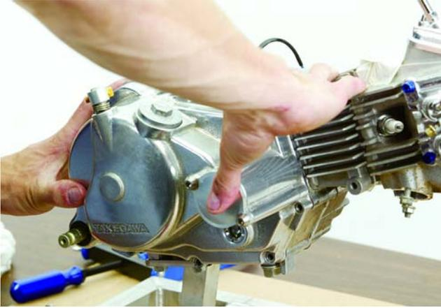
16. Tighten the clutch cover bolts to 7-8 ft. lbs.
