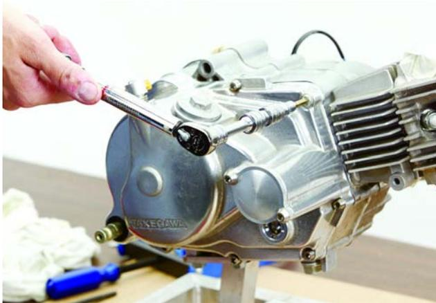
17. Add 850cc of engine oil. Double check the oil level using the sight window after the first start up. Add oil to proper level if needed. We recommend 10w40 synthetic motorcycle engine oil. ***DO NOT use any engine oil that contains moly.***
