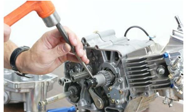
6. Remove the clutch center from the clutch assembly and install the clutch spacer in between the basket and the clutch center. The clutch spacer will ride on the bearing as shown.
