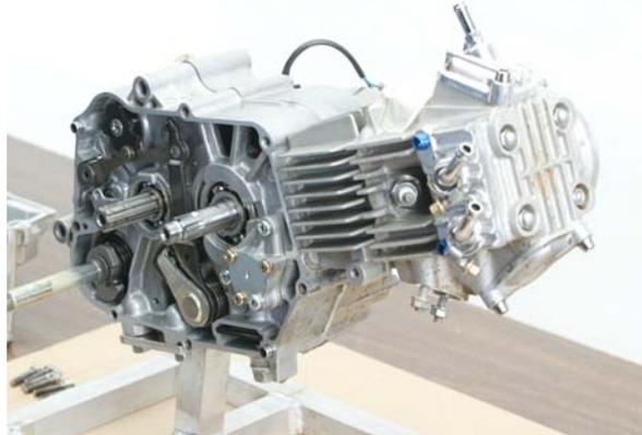
2. Make sure that the crankshaft spacer is installed over the crankshaft as shown. If you installed a stroke up kit and replaced the crank, the crankshaft spacer is probably still on the stock crank. Remove it and slide it over the crankshaft as shown along with the primary gear as shown.
