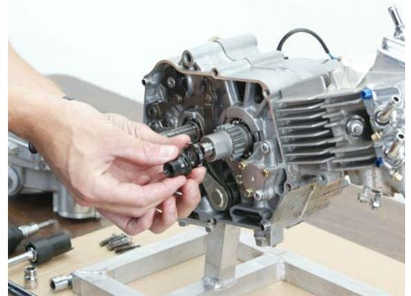
4. Tighten the clutch bearing to 29 ft. lbs.
