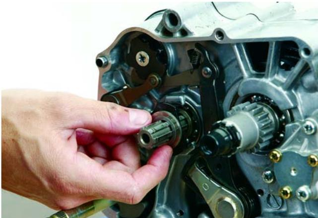
9. Be sure to liberally apply an assembly lubricant or engine oil to all parts, especially the bearing on both sides.
