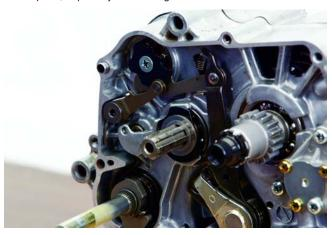
10. Slide the clutch assembly over the mainshaft. You may have to align the clutch spacer to get it over the shaft because it is "floating" in between the clutch center and the clutch basket.
