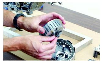
Note the order in which the bearing and spacers go over the clutch mainshaft.
