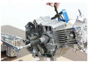
Using a hammer and a punch, gently fold over one of the tabs on the lock washer into the clutch bearing slot.
