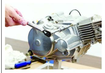
17. Add 850cc of engine oil. Double check the oil level using the sight window after the first start up. Add oil to proper level if needed. We recommend 10w40 synthetic motorcycle engine oil. <u>DO NOT use any engine oil that contains moly.</u>
