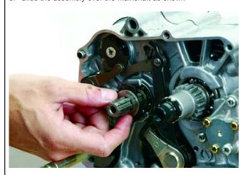
9. Be sure to liberally apply an assembly lubricant or engine oil to all parts, especially the bearing on both sides.
