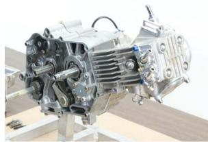
Make sure that the crankshaft spacer is installed over the crankshaft as shown. If you installed a stroke up kit and replaced the crank, the crankshaft spacer is probably still on the stock crank. Remove it and slide it over the crankshaft as shown along with the primary gear as shown.
