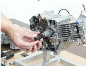
4. Tighten the clutch bearing to 29 ft. lbs.
