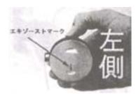
("R" mark is the top ring, "RN" mark is second from top) Install piston rings (bottom ring first) referencing the diagram.
