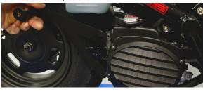
Install TBR Header pipe using the OEM gasket between header pipe and cylinder head, use OEM bolts.
