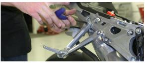
26. Replace tail light assembly, reconnect wiring and replace rear cowling, passenger & driver seats.
