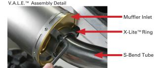
Attach the X-Lite<sup>™</sup> V.A.L.E.<sup>™</sup> assembly to the muffler canister using the 4 (four) 6mm x 14mm socket head cap screws. Leave loose for now.
