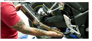
Mount muffler to mounting bracket using supplied hardware.
