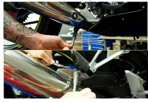
Install supplied muffler mount to right side rear foot peg using OEM bolt and nut.
