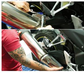
Install supplied muffler mount to right side rear foot peg using OEM bolt and nut.
