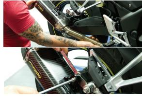
Double check all work for proper fit and alignment. Make sure all fasteners are tight.
