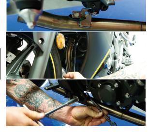
12. Install O2 sensor and plug into OEM wiring harness.
