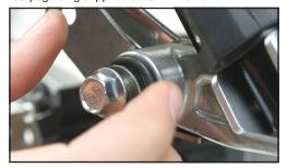
4. Attach muffler to TBR slip system using the supplied X-ring, 8x20mm socket head cap screws and lock washers that are provided, leave loose for now. Slide rubber lined muffler clamp and barrel clamp on and install to bike.
