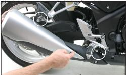
Install supplied muffler mount to right side rear footpeg using supplied 6x45mm bolt and nut.
