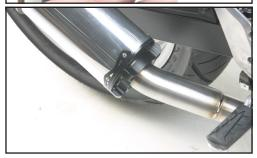
Loosely attach muffler to bike using the 8x35mm bolt and nut and install muffler clamp to outside of TBR mount.
