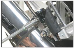
Check for clearance and alignment, then tighten all the bolts in this order: X-ring bolts, muffler mount, and finally barrel clamp.
