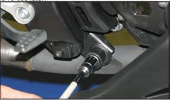
5. Remove header flange nut and remove header pipe.
