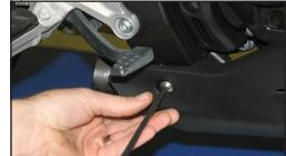
Remove header mounting bracket hardware, save to re-use later.
