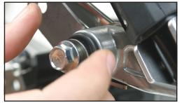
Attach muffler to TBR slip system using the supplied X-ring, 8x20mm socket head cap screws and lock washers that are provided, leave loose for now. Slide rubber lined muffler clamp and barrel clamp on and install to bike.
