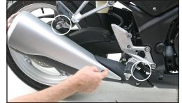
Remove rear right fairing mount to access header pipe bolt.
