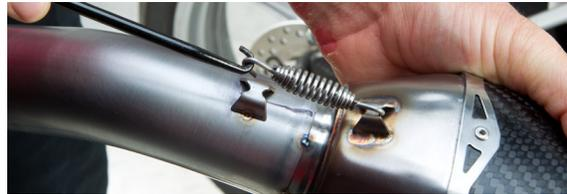
4. Install TBR slip-on assembly onto stock header and attach muffler bracket to passenger peg mount using supplied bolt, washer, and nut. Tighten to snug.
