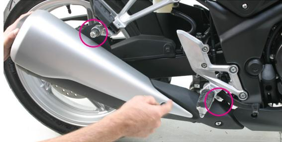
3. Apply a thin layer of anti-seize to TBR slip tube outlet and connect to Tarmac muffler using supplied hook springs. Loosely install barrel clamp onto slip tube inlet.
