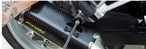
5. Tighten barrel clamp at header connection.
