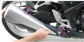
Apply a thin layer of anti-seize to TBR slip tube outlet and connect to Tarmac muffler using supplied hook springs. Loosely install barrel clamp onto slip tube inlet.
