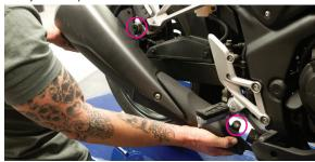
4. Remove header mounting hardware, save to re-use later.
