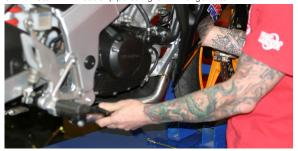
6. Install TBR slip-tube and supplied barrel clamp.
