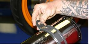
Loosely attach muffler to bike using the 8x50mm bolt, nut, spacer, and install muffler clamp to outside of mount.
