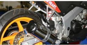
permanent when the system gets hot. Run the bike and enjoy. It is normal for some white smoke to appear the first time you start the bike. This is packing/manufacturing oil from inside the pipe burning off. Check for gaps or leaks. If you find a leak, a little high temperature silicon sealant should fix it. After 50 to 100 miles, recheck all fasteners for tightness.
