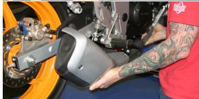
Install TBR header pipe using OEM flange nuts.
