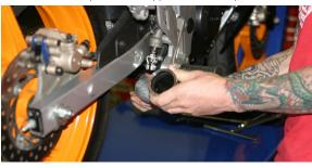
Attach muffler to TBR slip system using the supplied X-ring, 8x20mm socket head cap screws and lock washers that are provided, leave loose for now. Slide rubber lined muffler clamp and barrel clamp on and install to bike.
