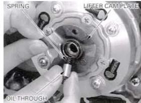
4. Remove the four bolts holding the clutch plate. Under this plate is the clutch locknut. Peel back the tab(s) on the lock washer. Remove this nut using either a Honda clutch locknut wrench or the Takegawa clutch locknut wrench (Part # 010-9-01-021, \$26.98 MSRP). A flywheel holder tool may help to remove this part.
