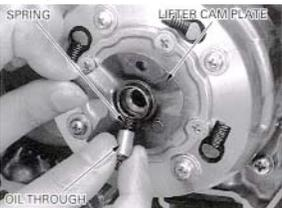
18. Reinstall the ball retainer and spring. Reinstall the clutch lifter lever.
