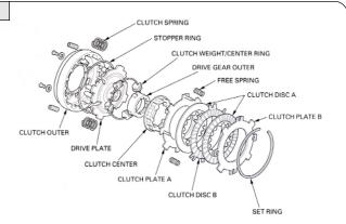
Remove the four phillips head screws and washers (photo A). Please not the once removed the four damper springs will drop down (photo B). Turn clutch assembly over and remove drive plate assembly and clutch springs (photo C).
