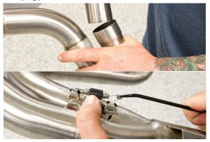
12. Install TBR system onto motorcycle. Leave cylinder nut slightly loose.
