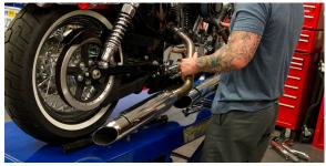
Remove O2 sensors to install on TBR head pipes.
